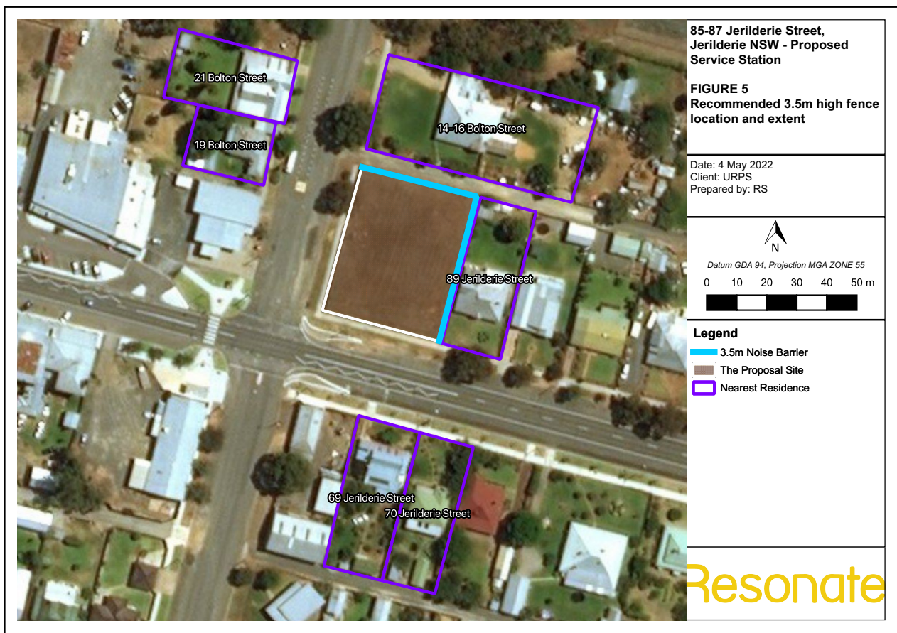
Figure 5: Recommended 3.5m high noise fence
