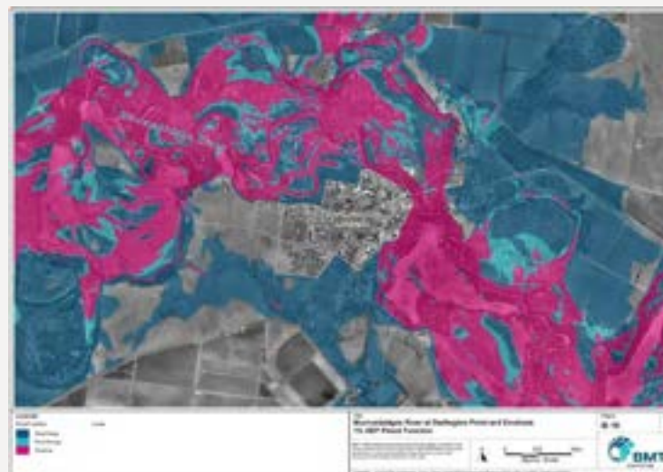
Figure 35: 1 in 100 Year Flood Map – Hydraulic Categories for Darlington Point (Source: Murrumbidgee River at Darlington Point Flood Study, 2018)
