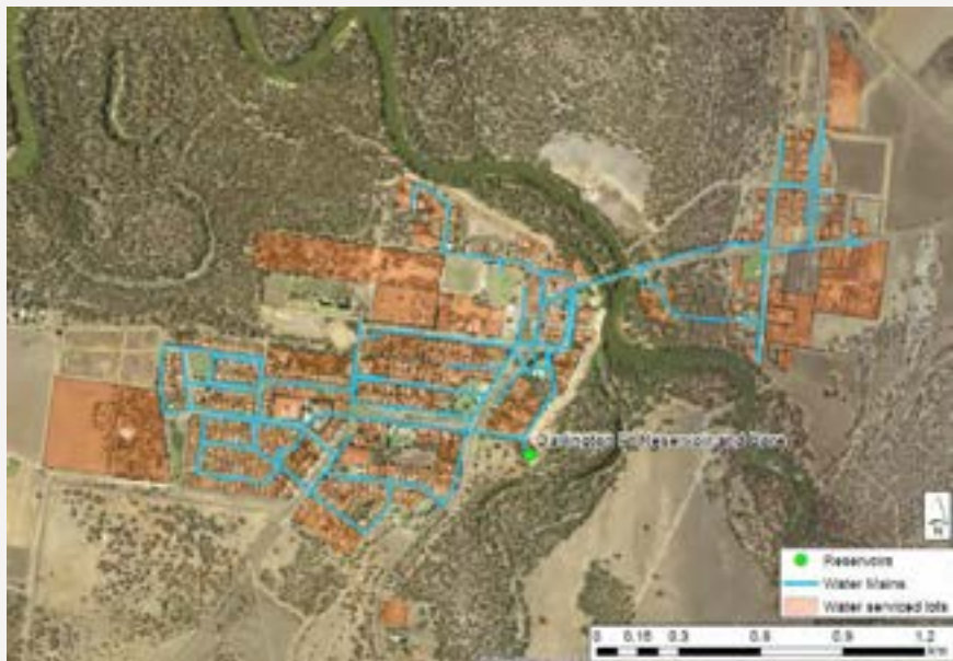
Figure 39: Darlington Point water supply scheme distribution map (Source: Draft Integrated Water Cycle Management Strategy)
