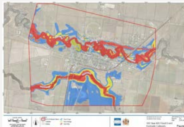
Figure 63: 1 in 100 Year Flood Map – Hydraulic Categories for Jerilderie (Source: Jerilderie Flood Study, 2014)
