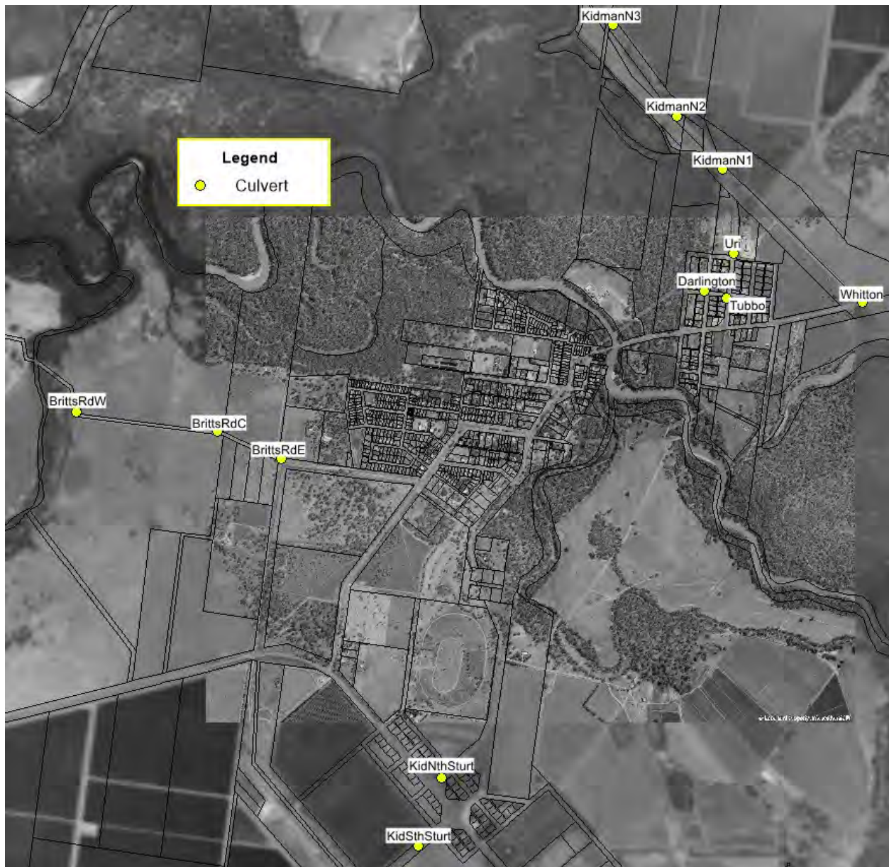
Plate C. 2 - Culvert updates included in the TUFLOW model as part of the updates in the 2020 Flood Study
