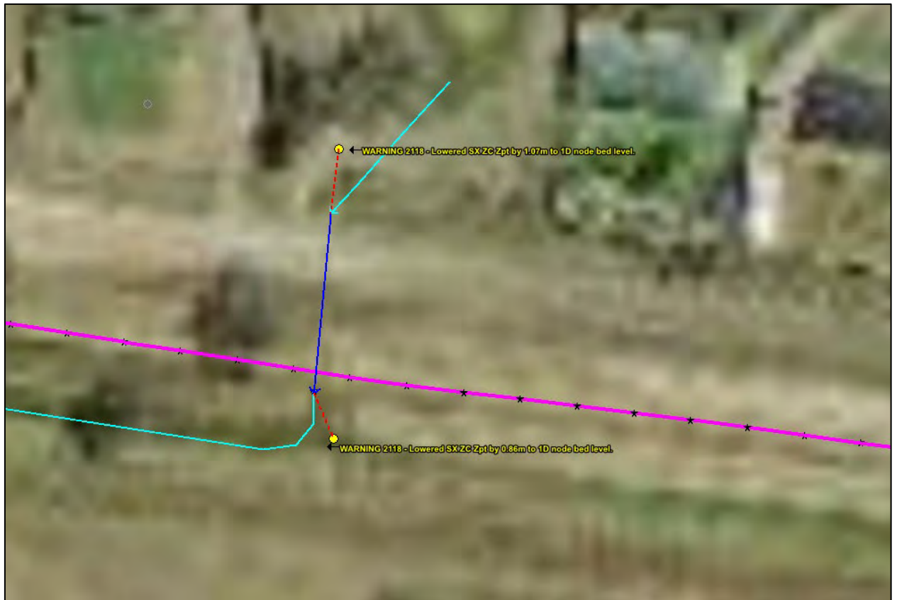
Plate 4 Example of 1D/2D connections at a levee cross-drainage structure (SX point shown as a yellow dot, CN as a red dashed line, culvert as a dark blue arrow, gully line in aqua and model warnings in yellow text)
