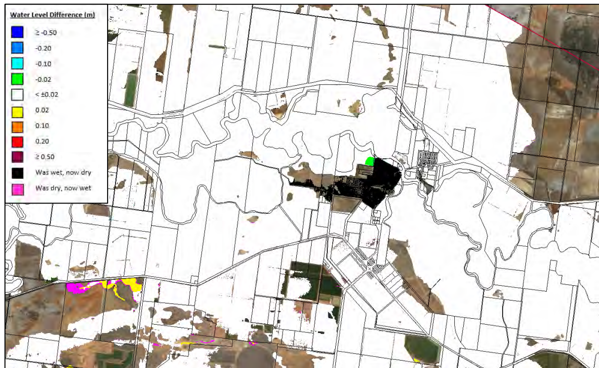
Plate H.16 – FM Option 3 (with a 100m wide spillway) floodwater level differences for the 0.2% AEP
