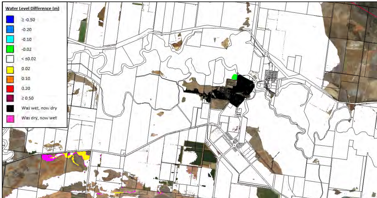
Plate H.14 – FM Option 3 (with a 200m wide spillway) floodwater level differences for the 0.2% AEP
