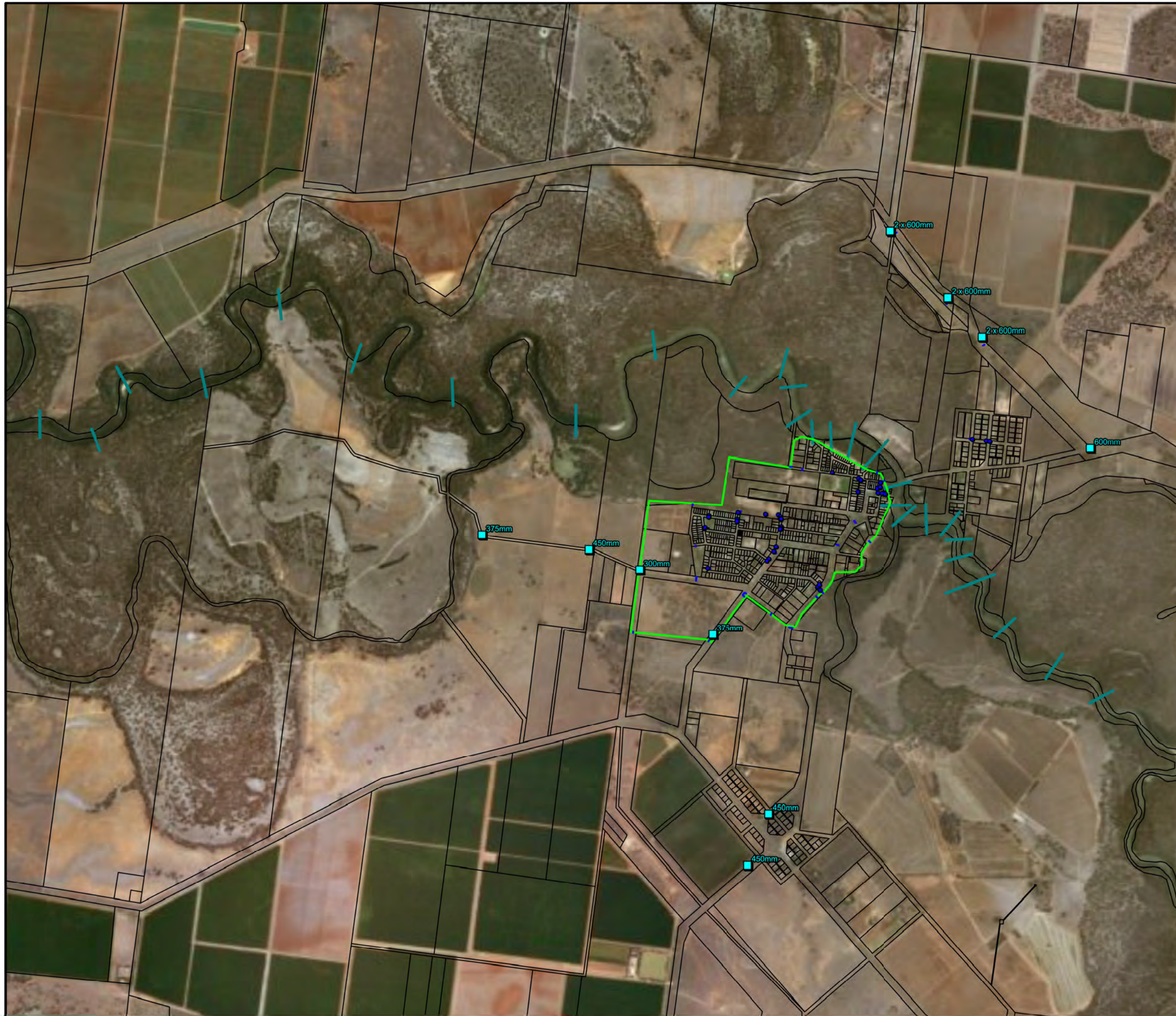
Figure 10: Stormwater Pipe Network of Local Darlington Point Study Area
