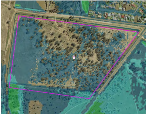
Plate E.5: Site 2 - 1%AEP design flood event hazard
