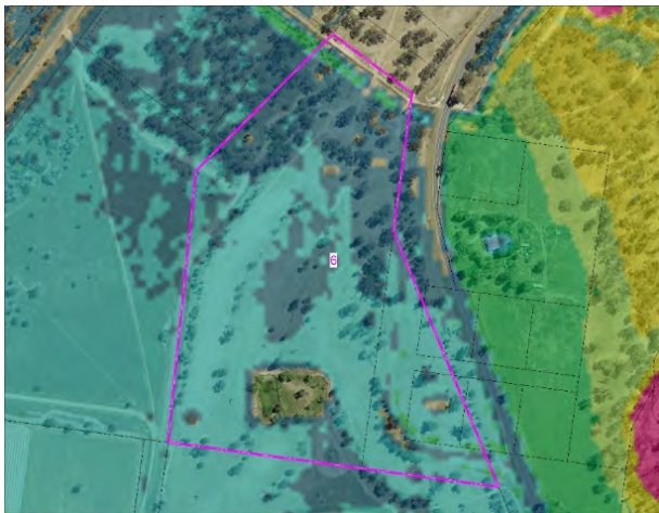
Plate E.13: Site 6 - 1%AEP design flood event hazard
