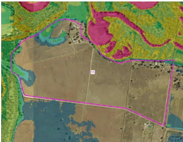
Plate E.25: Site 11 - 1%AEP design flood event hazard
