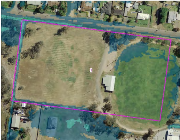
Plate E.3: Site 1 - 1%AEP design flood event hazard
