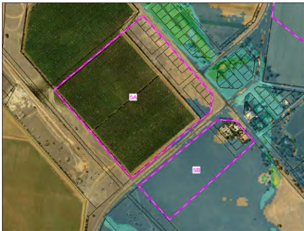
Plate E.11: Site 5 - 1%AEP design flood event hazard
