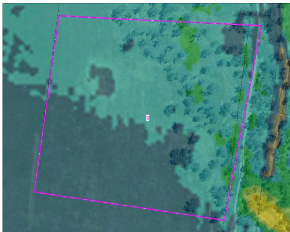
Plate E.19: Site 9 - 1%AEP design flood event hazard
