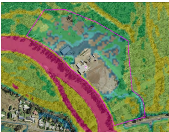
Plate E.15: Site 7 - 1%AEP design flood event hazard
