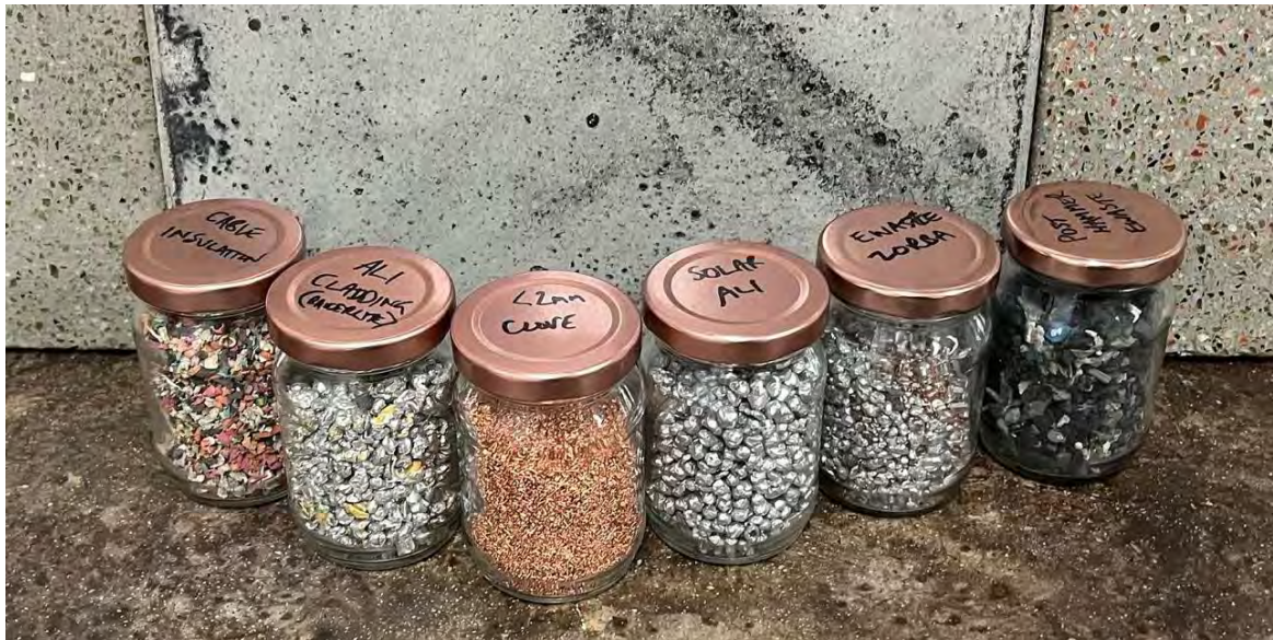
Cable insulation and other solar farm components after recycling
